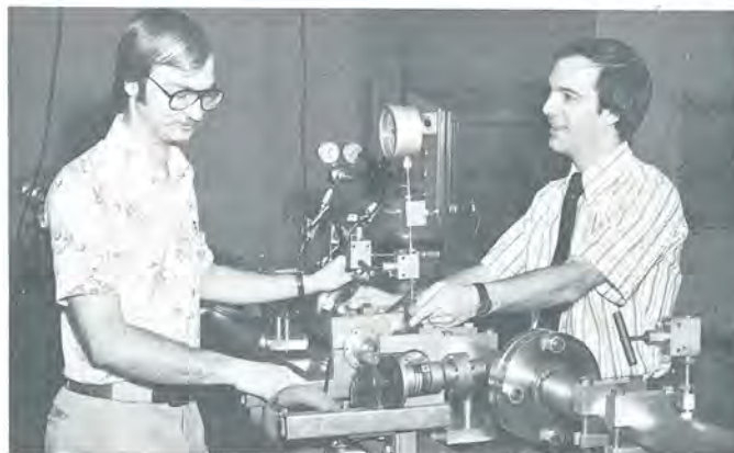
Dr. Thomas W. Lester (right) and his graduate student in nuclear engineering, Randy Seeker , are using this recently-installed shock tube to study the combustible properties of coal. The suspension of pulverized coal in a shock tube and the temperature and heating rate of coal closely resemble that in a furnace.
