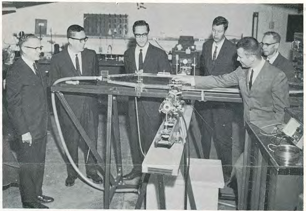
DEMONSTRATING A TEST SET-UP used to study flow bi-refringence in a current engineering research project is Dr. Richard Akins, associate professor of chemical engineering (right foreground). Faculty members of the department of chemical engineering observing the demonstration include, from left, Dr. William Honstead, department head; Dr. L. T. Fan, professor; Dr. John C. Matthews, assistant professor; Dr. Benjamin G. Kyle, professor; and Dr. Herbert T. Bates, professor.
