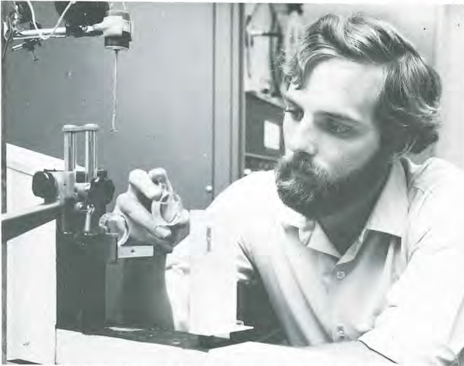
Jon Held, graduate student in Mechanical Engineering, holds a calibration cell containing a known particle size distribution and concentration used to test the accuracy of the instrument he
