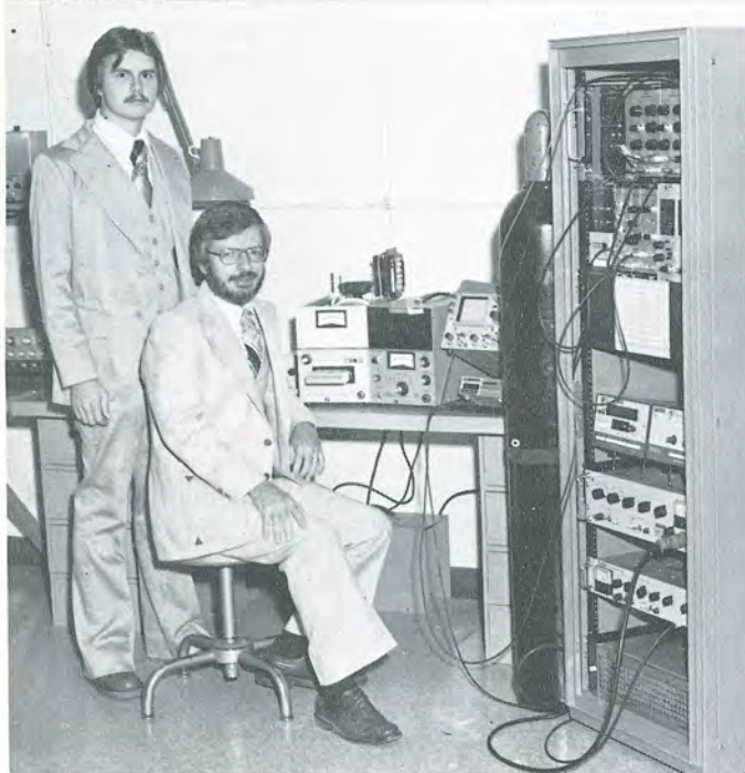
Researchers at K-State are studying thermoluminescent dosimetry (TLDs), a method of detecting and measuring the energy imparted per unit mass to matter by the interaction of radiation. Pictured are Don Hanna, graduate student, and Dr. Gale Simons, associate professor of Nuclear Engineering with the photon counter used to study the TLDs.
