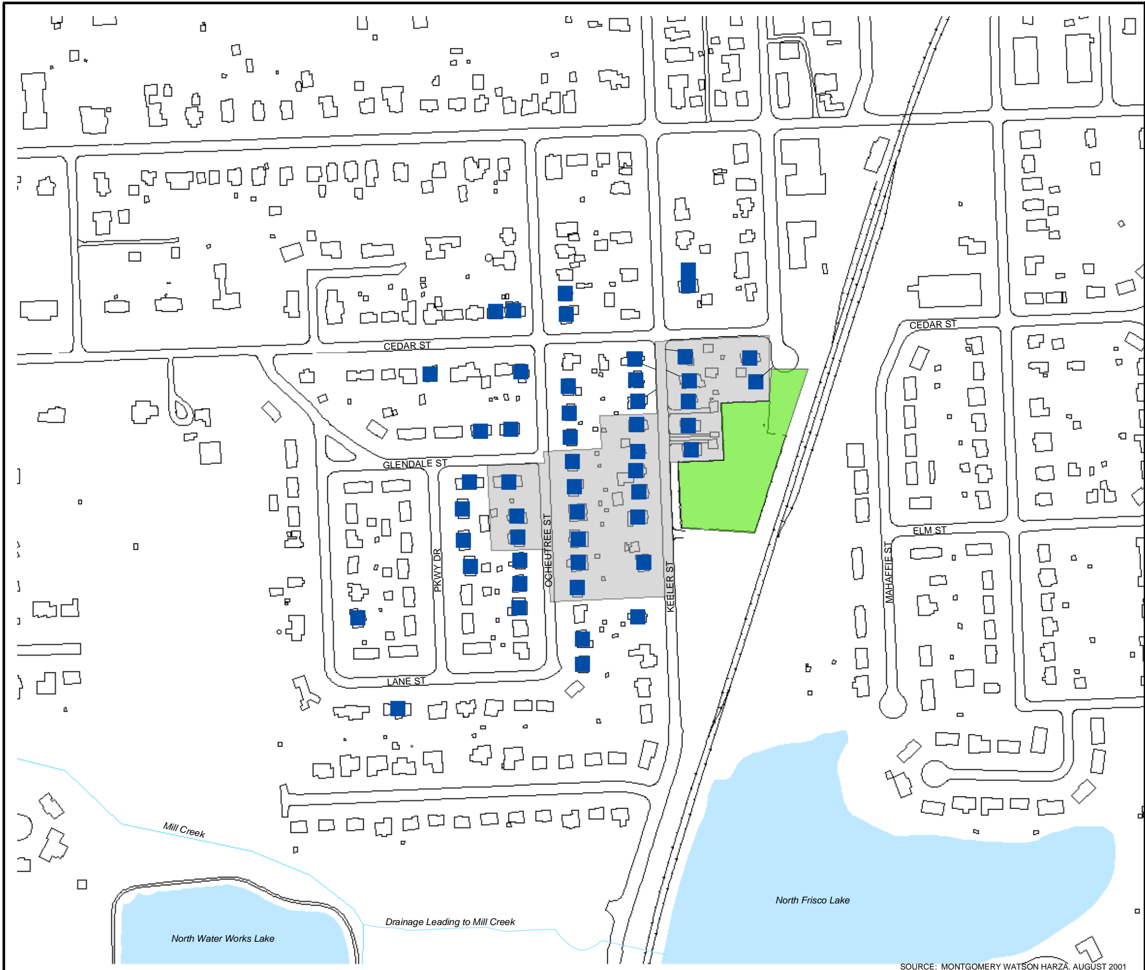
FIGURE 1 CCI SITE, GROUNDWATER TCE PLUME, AND PROPERTIES INCLUDED IN AIR SAMPLING PROGRAM
