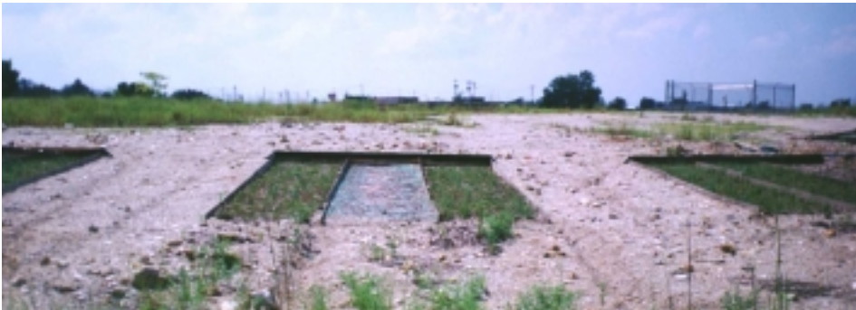
Phytostabilization of mine spoils ( chat ) in Galena, Kansas. Without revegetation, wind and rain can spread heavy metals beyond initial site of contamination. From Lambert, et al., 1999).
