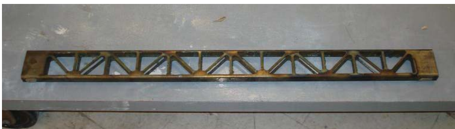
A piece of the bridge deck after being plasma cut.
